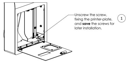
Remove the printerplate and **save** for later installation.
