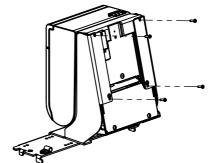
3 Insert printer plate into part A and fasten it with the saved screw from step 2.
