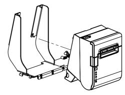
Mount the Printer with 4x Pan head K30x12mm.
