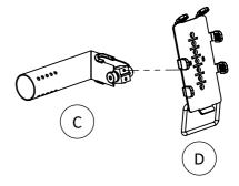
Mount Part C and Part D together using 2x Hex socket flat countersunk M4x10mm.
