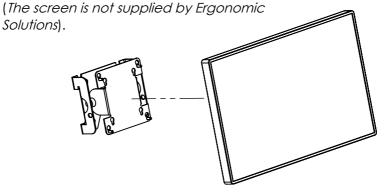
Mount the screen onto the VESA plate with 4x Pozi pan head M3x6mm.
